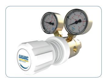
The Tech Master GPT410 Series two stage diaphragm cylinder regulators are designed for primary pressure gas control of technical grade Acetylene gas up to 4.5 purity (99.995%), on applications where constant delivery pressure is required as the cylinder pressure decreases.
