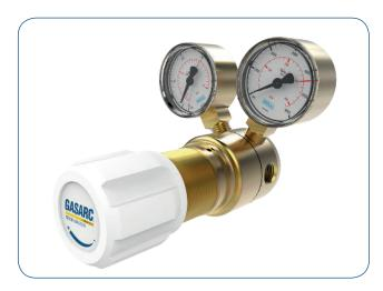
The Tech Master GPS420 Series single stage piston cylinder regulators are designed for primary pressure gas control of non-corrosive or toxic, technical grade gases up to 4.5 purity (99.995%), on applications where slight pressure variation from decreasing cylinder pressure is acceptable.
