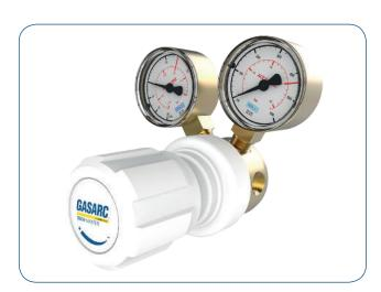
The Tech Master GPS410 Series single stage diaphragm cylinder regulators are designed for primary pressure gas control of technical grade Acetylene gas up to 4.5 purity (99.995%), on applications where slight pressure variation from decreasing cylinder pressure is acceptable.
