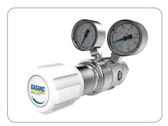
The Spec Master HPT620 Series two stage piston cylinder regulators are designed for primary pressure gas control of non-corrosive or toxic, high purity gases up to grade 6.0 purity (99.999%), on applications where constant delivery pressure is required as the cylinder pressure decreases.
