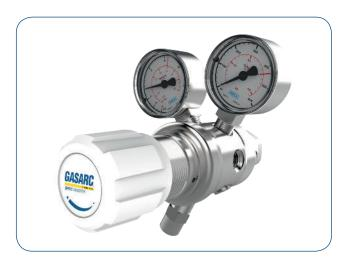
The Spec Master HPT600 Series two stage diaphragm cylinder regulators are designed for primary pressure gas control of non-corrosive or toxic, high purity gases up to grade 6.0 purity (99.9999%), on applications where constant delivery pressure is required as the cylinder pressure decreases.
