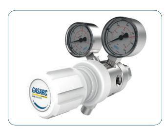
The Lab Master LGT500 Series two stage diaphragm cylinder regulators are designed for primary pressure gas control of non-corrosive or toxic, high purity gases up to grade 5.0 purity (99.999%), on applications where constant delivery pressure is required as cylinder pressure decreases.
