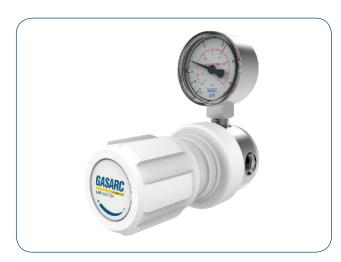
The Lab Master LGL510 Series single stage diaphragm line regulators are designed for secondary pressure gas control of high purity Acetylene gas up to grade 5.0 purity (99.999%), on gas distribution systems.
