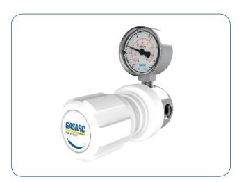
The Lab Master LGL500 Series single stage diaphragm line regulators are designed for secondary pressure gas control of non-corrosive or toxic, high purity gases up to grade 5.0 purity (99.999%), on gas distribution systems.
