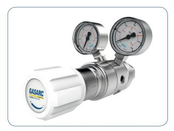
The Chem Master SGT620 two stage piston cylinder regulators are designed for primary pressure gas control of corrosive, toxic and high purity gases up to grade 6.0 purity (99.9999%), on applications where constant delivery pressure is required as the cylinder pressure decreases.
