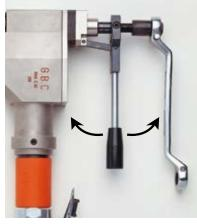
Lever handle for feeding the cutter head in tight spots where manual feeding is impossible.
