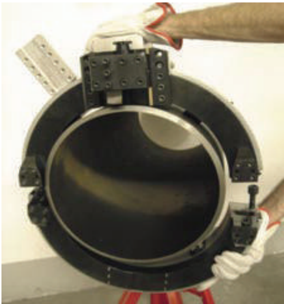
Developed for on site use in pipelines, machine body is split frame type allowing set up of machine at any point along pipelines.
