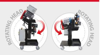
The machine is equipped with a stepless variable head type which allows bevel angles from 10° to 70°, granting a very easy and quick adjustment of the angle of bevel.
