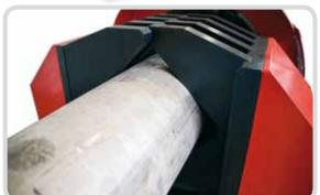
at the same time user friendly. The locking vice design enables the automatic centring and positioning without causing deformation to the pipe.
