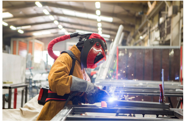
An example of personal fume extraction
