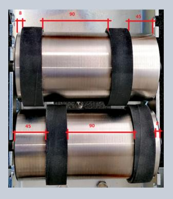
Place the ring next to the location where it is to be glued. Spread glue on the roller and rubber ring, and let dry for 5 – 10 minutes. Turn over the rubber ring onto the glued area so that the two glued surfaces are in contact with each other.
