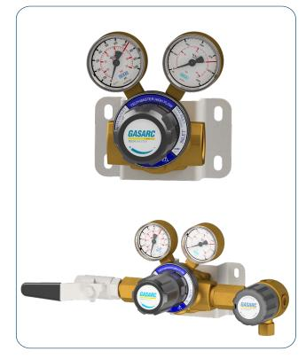
The Tech Master D1G High Flow Regulator is uniquely designed with both a dome loaded and pilot regulator built into a single compact unit. Bringing the benefit of a consistent flow rate intended for High Flow applications (up to 500m3/hr @ 125bar inlet pressure). Typical examples; laser cutting, fire suppression and gas purging. Available in both a regulator and control panel format, control panel is fitted with a high flow valve and a ball valve.
