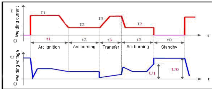
Current and Voltage Changes in DC MMA
