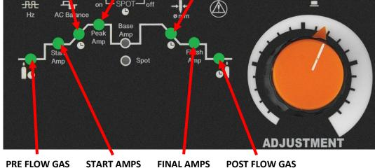
Set parameters as follows using control panel image above as reference:
