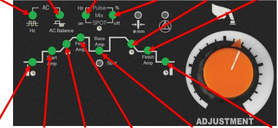
PRE FLOW GAS START AMPS UPSLOPE WELDING AMPS BACKGROUND CURRENT POST FLOW GAS
