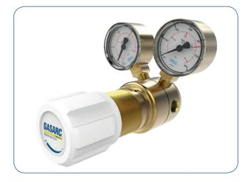
The Tech Master GPS420 Series single stage piston cylinder regulators are designed for primary pressure gas control of non-corrosive or toxic, technical grade gases up to 4.5 purity (99.995%), on applications where slight pressure variation from decreasing cylinder pressure is acceptable.
