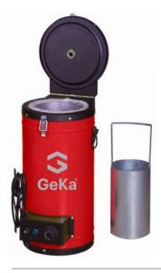
Its main function is to help keep electrodes manually at the desired temperature level between 60 and 200°C at the points of application. It can easily be used with all types of electrodes.
