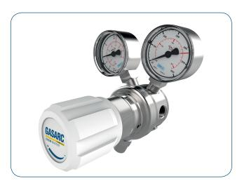
The Chem Master SGS600 single stage diaphragm cylinder regulators are designed for primary pressure gas control of corrosive, toxic and high purity gases up to grade 6.0 purity (99.9999%), on applications where slight pressure variation from decreasing cylinder pressure is acceptable.
