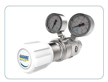
The Spec Master HPT620 Series two stage piston cylinder regulators are designed for primary pressure gas control of non-corrosive or toxic, high purity gases up to grade 6.0 purity (99.999%), on applications where constant delivery pressure is required as the cylinder pressure decreases.
