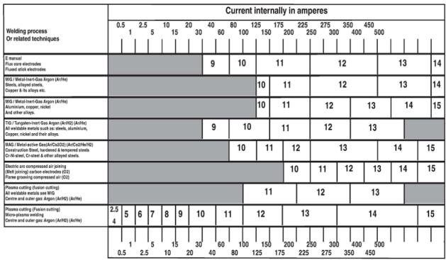
Depending upon the application conditions, the next highest or next lowest protection level can be used. The darker fields correspond to those areas in which the corresponding welding process cannot be used.
