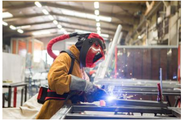
An example of personal fume extraction
