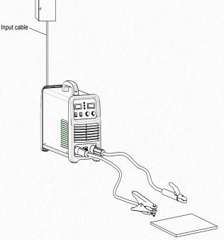
socket on the front panel of the welding machine, and tighten it clockwise
