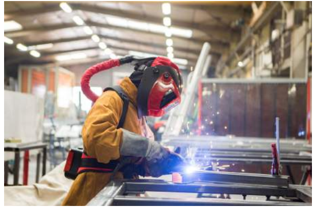
An example of personal fume extraction
