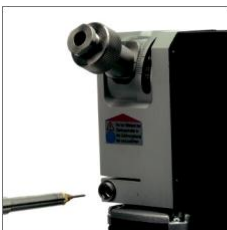
Precise adjustment of the electrode's stick-out.
